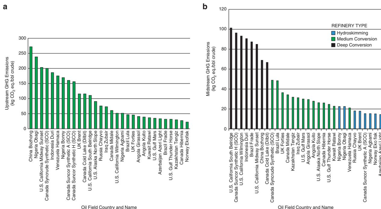
Figure 3 GHG emissions for 30 oils at upstream (oil production) (a) and midstream (refinery) (b) stages<sup>10</sup>: Gordon et al., 2015.
