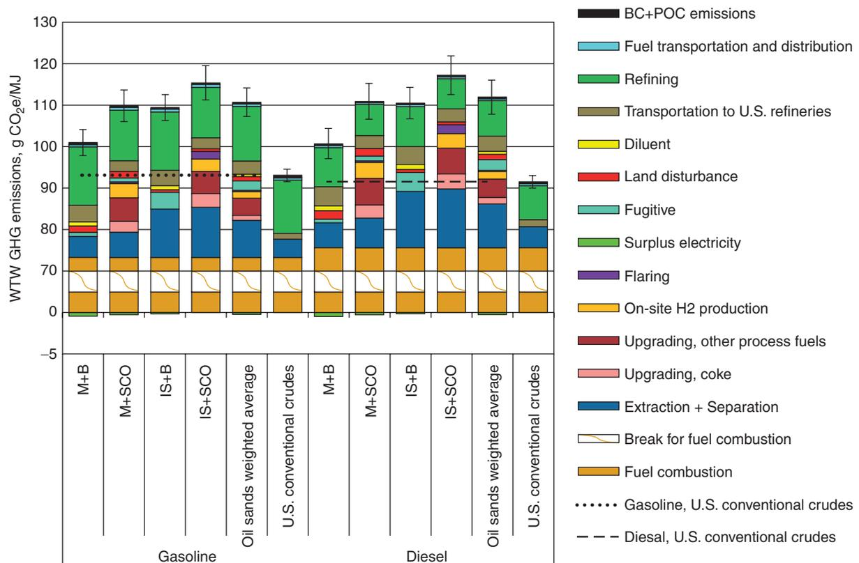
Figure 2 WTW GHG emissions of gasoline and diesel. Source: Cai et al. (2015). See reference for explanation of basis for vertical bars. (M, Mining; B, bitumen; SCO, synthetic crude oil; IS, in situ).
